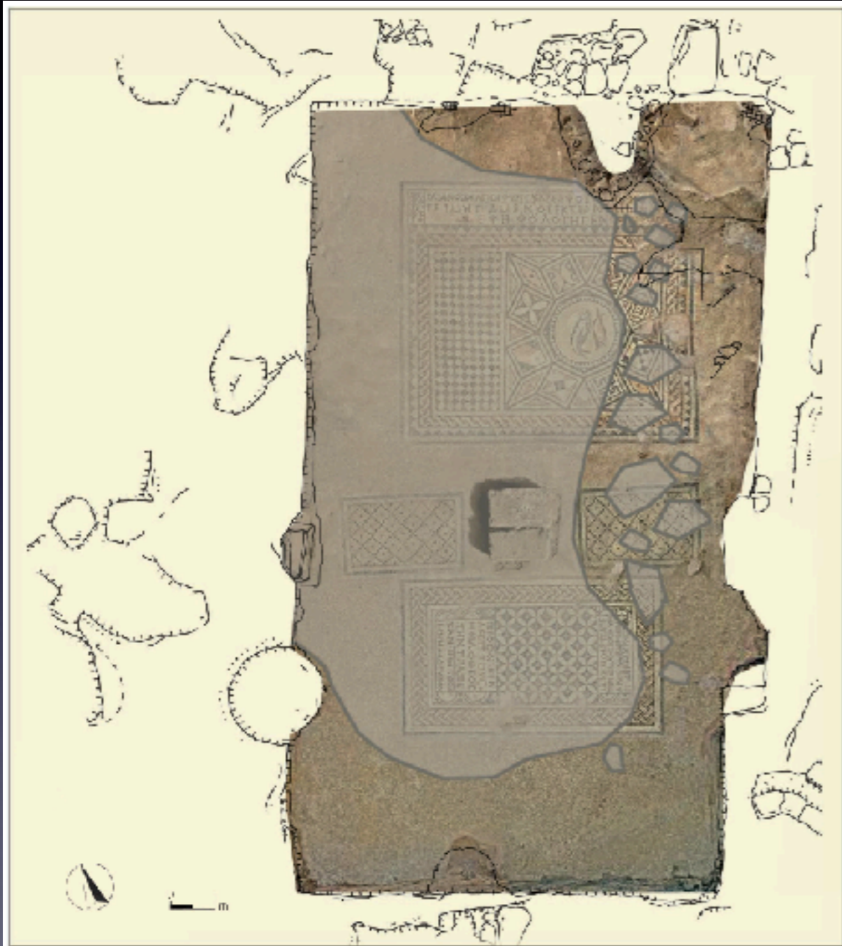
Plan illustrating the layer of plaster (in grayish-brown) covering the mosaic floor.
